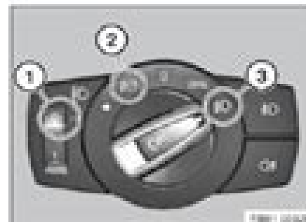
Fig. 15. Identifying Low Beam/Driving Light Position
