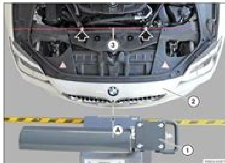
Fig. 16. Positioning Headlight Adjustment Device
