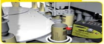
Objective: To detect registration marks on tubes for correct positioning before filling.
