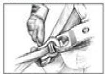
Secure to the anchor point with a tree trunk protector or choker chain. Attach the clevis/shockle. Attach the shaddle to the two ends of the strap! chain, being careful not to over tighten (tighten and back off 1/2 turn).
