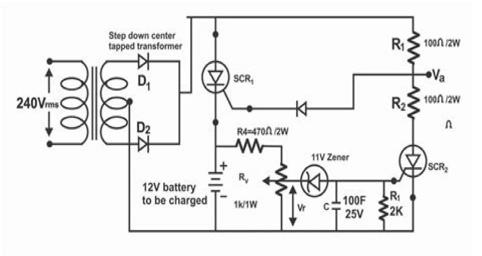
Fig 6.30 A battery charger using two SCRs
