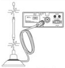
Connect the antenna cable plug to the receptacle marked "ANT" on the back of the unit.
