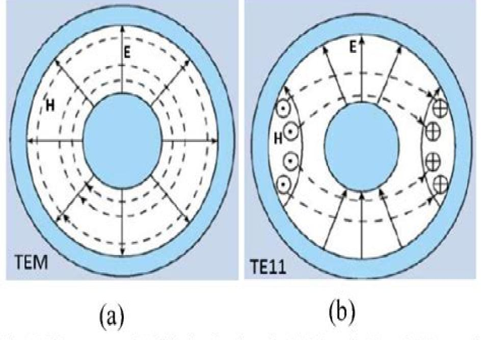
Fig. 5. Electromagnetic field distributions for TEM mode (a) and TE<sub>11</sub> mode
