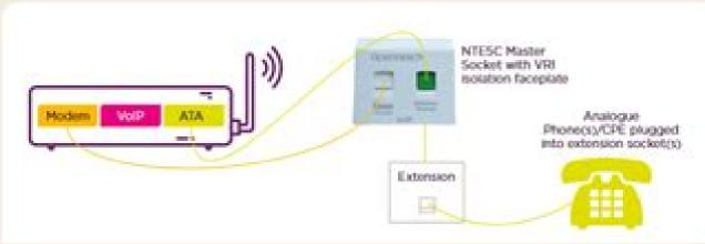
SOGEA plus ATA derived voice over extension wiring and isolated VRI
