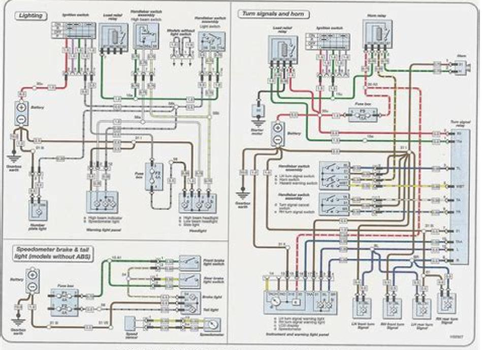
R1100 S ('01 onwards) : Lighting, speedometer, brake and tail lights, turn signals and hom
