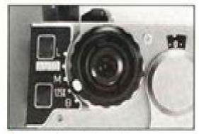
Load the film with the exposure mode dial set at "125X" and advance to the first exposure. (See page 8)
