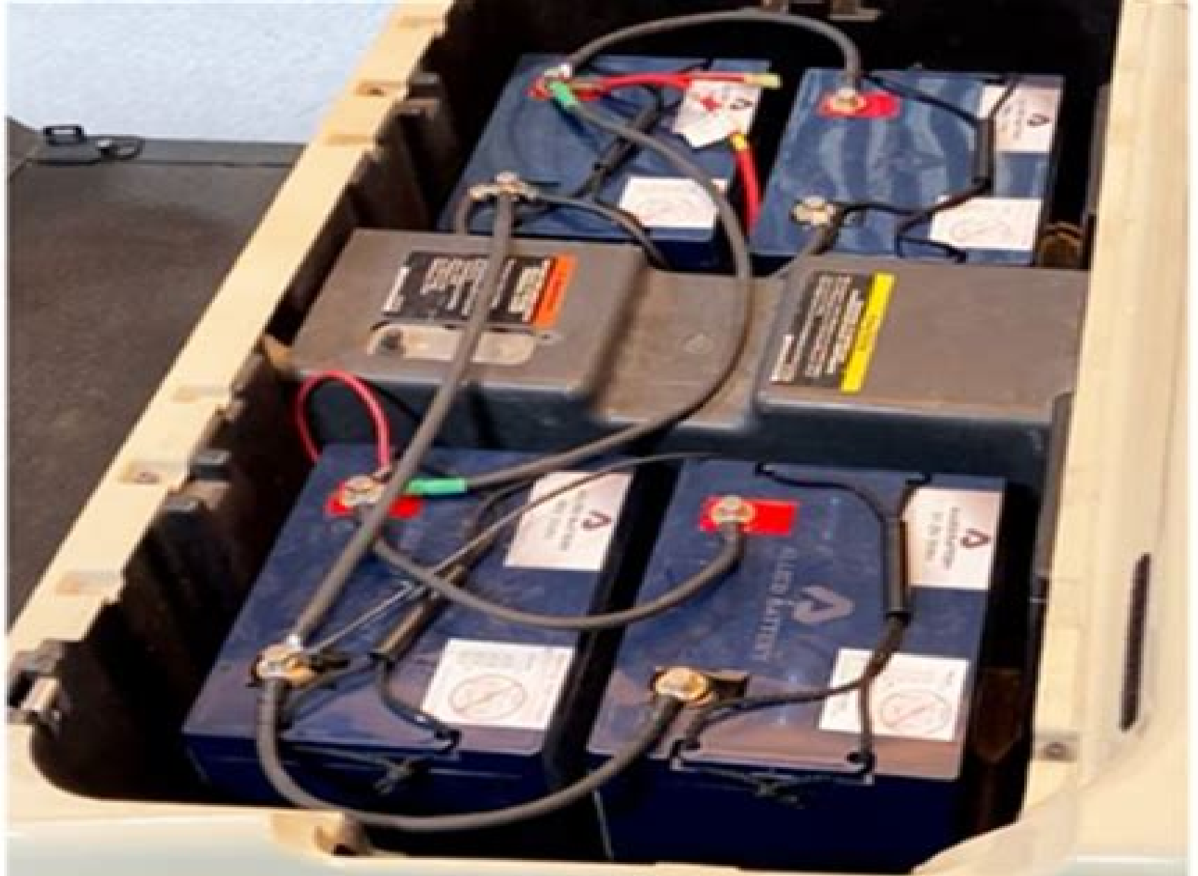
4 x 48V 30Ah (120Ah Setup)
