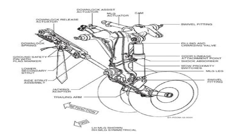
Main Landing Gear Assembly (LH Side Shown)
