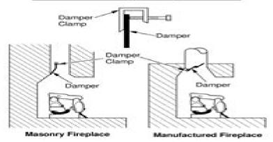
Figure 10 - Attaching Damper Clamp
