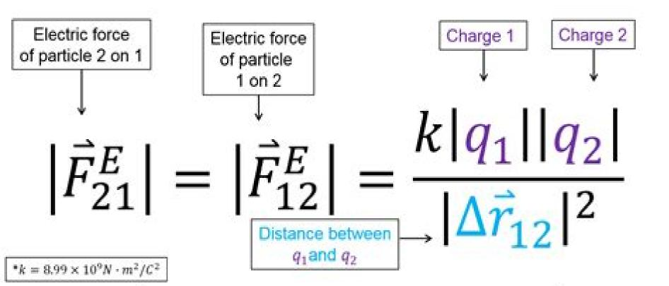
In words: The magnitude of the electric force of particle 2 on 1 is equal to the magnitude of the electric force of 1 on 2 which is equal to the constant k times the magnitude of  $q_1$ , times the magnitude of  $q_2$ , divided by the absolute distance between  $q_1$  and  $q_2$  squared
