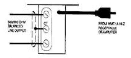
Figure 3 - Connecting WMT-1A as Output Meliching Transformer
