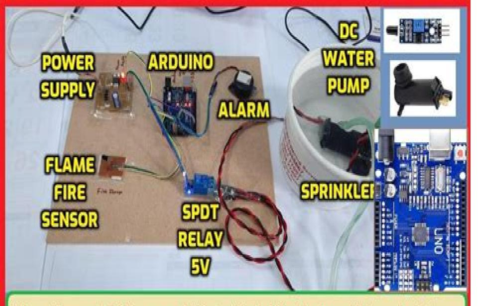
Fire Alarm with Siren and Water Sprinkler System Using Arduino
