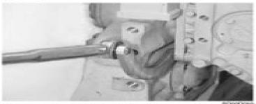
Using torque wrench adapter CAS-2754 remove the two bolts and washers on the front inside and the two bolts and washers on the rear inside of the final drive.
